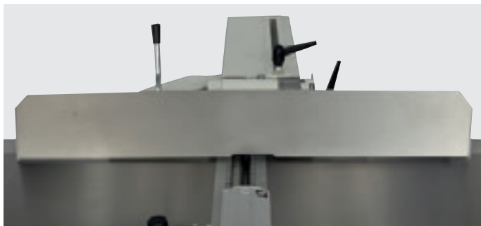
Tilting fence 90° ÷ 45° in ground cast iron.
