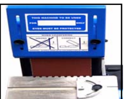
Thumb screw for the adjustment of belt
